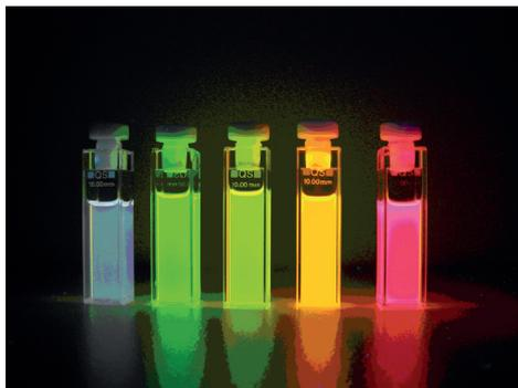
Fig. 1: Colloidal solutions of CdSe nanoparticles of different size
